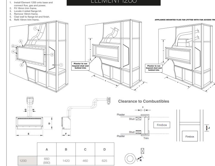
(880) for unit mounted fan. All measurements in millimetres (mm)
