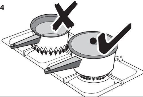
Make sure that the flames are under the pans. Using a lid will help the contents boil more quickly (**Fig. 2.4**).
