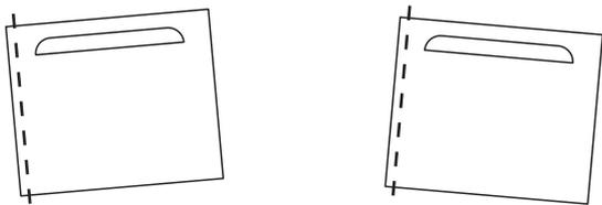
Effect of hinge adjustment – exaggerated for clarity
